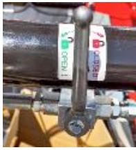
MANUAL LOCKING VALVE PREVENTING DESCENT ON LIFTING CYLINDER
